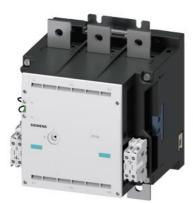
Contactor, Size 14, 3-pole, AC-3, 450 kW, 400/380 V (690 V) Auxiliary switch 44 (4NO+4NC) AC operation 230...276 V AC 50/60 Hz
