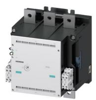
Contactor, Size 14, 3-pole, AC-3, 450 kW, 400/380 V (1000 V) Auxiliary switch 44 (4NO+4NC) AC operation 110...132 V AC 50/60 Hz
