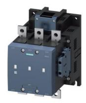
Vacuum contactor, AC-3 225 A, 110 kW / 400 V AC (50-60 Hz) / DC operation 220-240 V UC, Auxiliary contacts 2 NO + 2 NC, 3-pole, Size S10, busbar connections Drive: conventional
