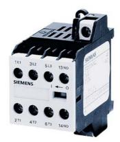
Power relay, AC-3 8.4 A, 4 kW / 400 V 3 NO+1 NC, 24 V DC 3 pole, screw terminal
