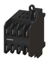
Power relay, AC-3 8.4 A, 4 kW / 400 V 3 NO+1 NC, 24 V DC 3 pole, flat connector terminal  $6.3 \times 0.8 \text{mm}$
