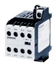
Power relay, AC-3 8.4 A, 4 kW / 400 V 4 NO, 110 V AC, 45...450 Hz 3 pole, screw terminal
