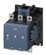
Vacuum contactor, AC-3 265 A, 132 kW / 400 V AC (50-60 Hz) / DC operation 110-127 V UC Auxiliary contacts 2 NO + 2 NC 3-pole, Size S10 Busbar connections Drive: conventional
