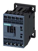
Contactor relay, 2 NO + 2 NC, 230 V AC, 50 / 60 Hz, Size S00, Spring-type terminal
