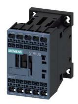
Contactor relay, 3 NO + 1 NC, 24 V AC, 50 / 60 Hz, Size S00, Spring-type terminal
