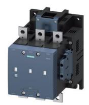
Vacuum contactor, AC-3 300 A, 160 kW / 400 V AC (50-60 Hz) / DC operation 110-127 V UC Auxiliary contacts 2 NO + 2 NC 3-pole, Size S10 Busbar connections Drive: conventional
