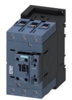
power contactor, AC-3 80 A, 37 kW / 400 V 1 NO + 1 NC, 24 V AC, 50 Hz 3-pole, 3 NO, Size S3 screw terminal
