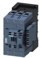
power contactor, AC-3 80 A, 37 kW / 400 V 2 NO + 2 NC, 110 V AC 50 Hz 3-pole, 3 NO, Size S3 Spring-type terminal
