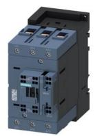
power contactor, AC-3 80 A, 37 kW / 400 V 1 NO + 1 NC, 230 V AC/50 Hz 3-pole, 3 NO, Size S3 Spring-type terminal
