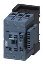
power contactor, AC-3 80 A, 37 kW / 400 V 2 NO + 2 NC, 230 V AC/50 Hz 3-pole, 3 NO, Size S3 Spring-type terminal
