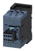
power contactor, AC-3 80 A, 37 kW / 400 V 2 NO + 2 NC, 24 V AC, 50 Hz 3-pole, 3 NO, Size S3 screw terminal
