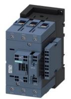
power contactor, AC-3 95 A, 45 kW / 400 V 2 NO + 2 NC, 230 V AC, 50 Hz 3-pole, 3 NO, Size S3 Spring-type terminal
