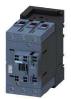
power contactor, AC-3 95 A, 45 kW / 400 V 1 NO + 1 NC, 220 V AC, 50 Hz 240 V/60 Hz 3-pole, 3 NO, Size S3 Spring-type terminal
