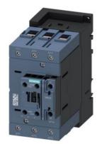
Contactor, AC-3, 55 kW/400 V 1 NO+1 NC, 110 V AC 50 Hz 3-pole, 3 NO, Size S3 Screw terminal
