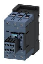
Power contactor, AC-3 110 A, 55 kW / 400 V 2 NO + 2 NC, 230 V AC, 50 Hz 3-pole, 3 NO, Size S3 screw terminal
