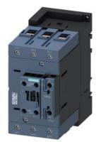
Power contactor, AC-3 110 A, 55 kW / 400 V 1 NO + 1 NC, 220 V AC, 50 Hz 240 V, 60 Hz 3-pole, 3 NO, Size S3 screw terminal
