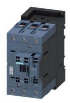
Contactor, AC-3, 55 kW/400 V 1 NO+1 NC, 110 V AC 50 Hz 3-pole, 3 NO, Size S3 Spring-type terminal
