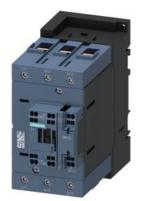
Power contactor, AC-3 110 A, 55 kW / 400 V 1 NO + 1 NC, 230 V AC, 50 Hz 3-pole, 3 NO, Size S3 Spring-type terminal
