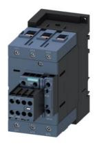
power contactor, AC-3 80 A, 37 kW / 400 V 2 NO + 2 NC, 230 V AC/50 Hz 3-pole, 3 NO, Size S3 screw terminal
