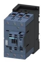
power contactor, AC-3 80 A, 37 kW / 400 V 1 NO + 1 NC, 24 V AC 50 Hz 3-pole, 3 NO, Size S3 Spring-type terminal
