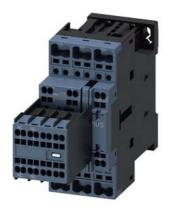
Contactor, AC-3, 15 kW / 400 V, 2 NO + 2 NC, 110 V AC, 50 Hz, 3-pole, Size S0 Spring-type terminal Removable auxiliary switch
