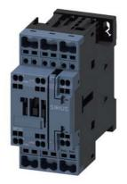
Power contactor, AC-3 38 A, 18.5 kW / 400 V 1 NO + 1 NC, 24 V AC 50 Hz, 3-pole, size S0 Spring-type terminals
