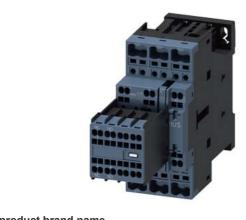
Power contactor, AC-3 38 A, 18.5 kW / 400 V 2 NO + 2 NC, 24 V AC 50 Hz, 3-pole, size S0 Spring-type terminals Removable auxiliary switch
