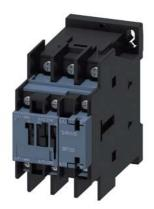
Power contactor, AC-3 38 A, 18.5 kW / 400 V 1 NO + 1 NC, 220 V AC 50 Hz, 240 V, 60Hz, 3-pole, size S0 ring cable lug connection
