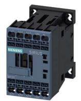
power contactor, AC-3 12 A, 5.5 kW / 400 V 1 NO, 220 V AC, 50 Hz 240 V, 60 Hz, 3-pole Size S00, Spring-type terminal
