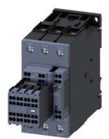
power contactor, AC-3 40 A, 18.5 kW / 400 V 2 NO + 2 NC, 110 V AC 50 Hz, 3-pole, Size S2, Spring-type terminal
