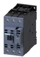
power contactor, AC-3 40 A, 18.5 kW / 400 V 1 NO + 1 NC, 220 V AC 50 Hz / 240 V, 60 Hz, 3-pole, Size S2, Spring-type terminal
