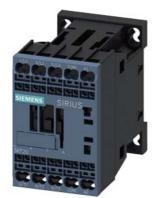
power contactor, AC-3 12 A, 5.5 kW / 400 V 1 NC, 220 V AC, 50 Hz 240 V, 60 Hz, 3-pole Size S00, Spring-type terminal
