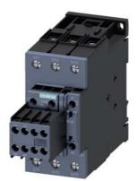
power contactor, AC-3 50 A, 22 kW / 400 V 2 NO + 2 NC, 110 V AC, 50 Hz, 3-pole, Size S2, screw terminal
