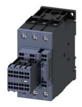
power contactor, AC-3 50 A, 22 kW / 400 V 2 NO + 2 NC, 110 V AC, 50 Hz 3-pole, Size S2, Spring-type terminal
