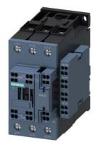
power contactor, AC-3 50 A, 22 kW / 400 V 2 NO + 2 NC, 110 V AC, 50 Hz 3-pole, Size S2, Spring-type terminal lateral auxiliary switch block
