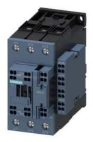
power contactor, AC-3 50 A, 22 kW / 400 V 2 NO + 2 NC, 230 V AC, 50 Hz 3-pole, Size S2, Spring-type terminal lateral auxiliary switch block
