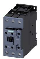
Contactor, AC-3, 30 kW / 400 V, 1 NO + 1 NC, 110 V AC, 50 Hz, 3-pole, Size S2, screw terminal
