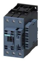
Power contactor, AC-3 65 A, 30 kW / 400 V 2 NO + 2 NC, 230 V AC, 50 Hz 3-pole, size S2 Spring-type terminals lateral auxiliary switch block
