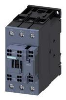
Power contactor, AC-3 65 A, 30 kW / 400 V 1 NO + 1 NC, 220 V AC, 50 Hz 240 V, 60Hz, 3-pole Size S2, Spring-type terminals
