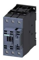
Contactor, AC-3, 37 kW / 400 V, 1 NO + 1 NC, 110 V AC, 50 Hz, 3-pole, Size S2, Spring-type terminal
