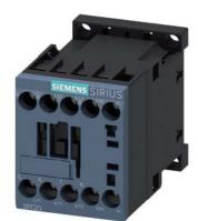
Power contactor, AC-3 16 A, 7.5 kW / 400 V 1 NC, 24 V AC, 50/60 Hz 3-pole, Size S00 screw terminals
