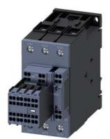
Contactor, AC-3, 37 kW / 400 V, 2 NO + 2 NC, 110 V AC, 50 Hz, 3-pole, Size S2, Spring-type terminal
