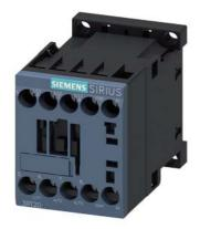
Power contactor, AC-3 16 A, 7.5 kW / 400 V 1 NC, 230 V AC, 50/60 Hz 3-pole, Size S00 screw terminals
