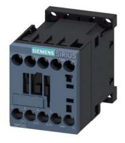
Power contactor, AC-3 16 A, 7.5 kW / 400 V 1 NO, 220 V AC, 50 Hz, 240 V 60Hz, 3-pole, Size S00 screw terminals
