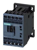
Contactor, AC-3, 7.5 KW / 400 V, 1 NC, 110 V AC, 50 / 60 Hz, 3-pole, Size S00 Spring-type terminal
