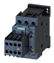
power contactor, AC-3 9 A, 4 kW / 400 V 2 NO + 2 NC, 230 V AC, 50 Hz 3-pole, Size S0 screw terminal Removable auxiliary switch
