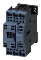
power contactor, AC-3 9 A, 4 kW / 400 V 1 NO + 1 NC, 230 V AC, 50 Hz 3-pole, Size S0 Spring-type terminal
