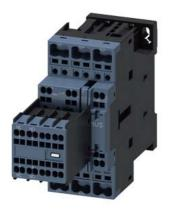
power contactor, AC-3 12 A, 5.5 kW / 400 V 2 NO + 2 NC, 110 V AC, 50 Hz 3-pole, Size S0 Spring-type terminal Removable auxiliary switch
