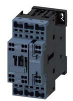
power contactor, AC-3 12 A, 5.5 kW / 400 V 1 NO + 1 NC, 220 V AC, 50 Hz 240 V, 60 Hz, 3-pole Size S0, Spring-type terminal
