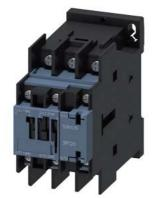
power contactor, AC-3 12 A, 5.5 kW / 400 V 1 NO + 1 NC, 220 V AC, 50 Hz 240 V, 60 Hz, 3-pole Size S0 ring cable lug connection
